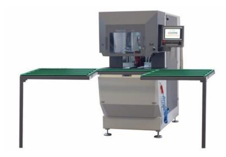
TORNADO CNC Computer Numerically Controlled corner cleaning machine is designed for PVC frames and
