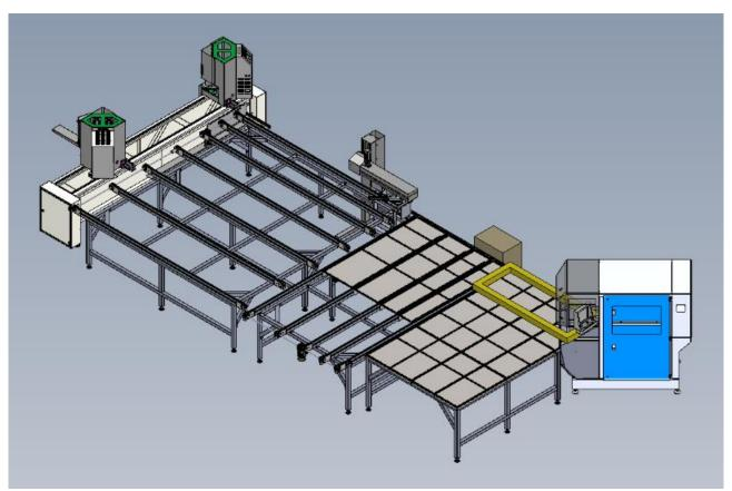
The corner welding and cleaning line for PVC profiles AUSTER consists of 5 main parts and depending on the welding machine installed in the line can handle frames of various sizes, in a fully automated mode:
